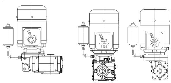
Figure 19: Position of the oil expansion chamber
