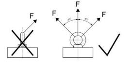
Only use the eyebolts attached to the gear unit for transport. If geared motors have an additional eyebolt attached to the motor, this must also be used.
