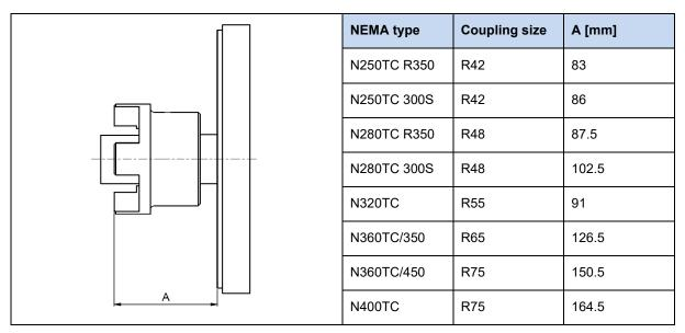
Table 8: Position of the half-coupling on the NEMA motor shaft
