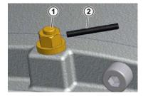
Figure 21: Activating the pressure vent screw
