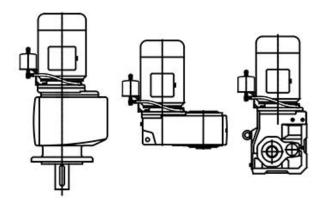
Figure 18: Position of the oil expansion chamber
