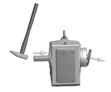
Figure 5: Removing the factory-fitted closing cap
