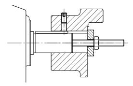
Figure 2: Example of a simple pulling device
