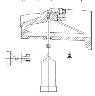
Figure 23: Fitting the grease collection container
