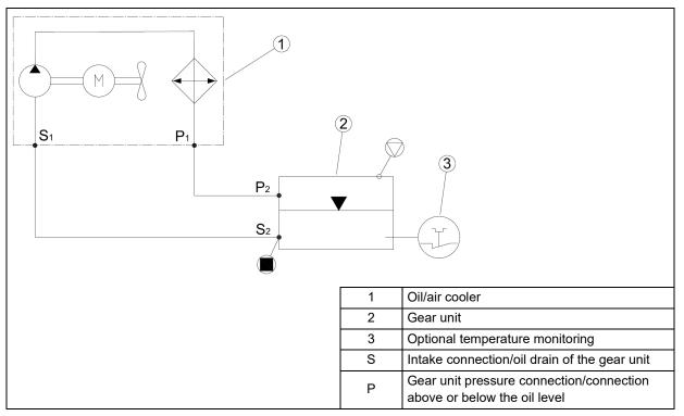
Figure 17: Connection of the oil/air cooler
