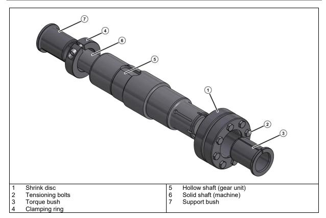
Figure 12: GRIPMAXX™, exploded diagram
